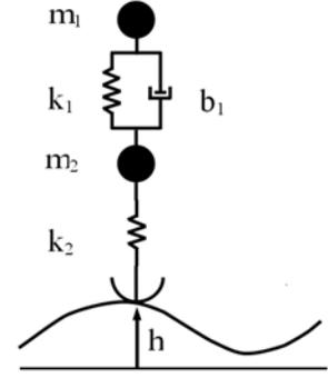
Figure 3: Quarter model of a vehicle
