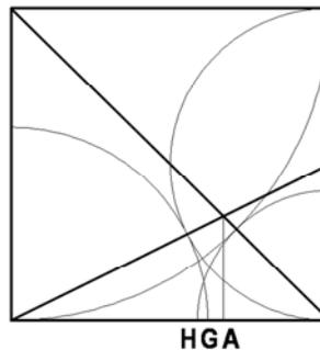
Figure 3: Division of a line segment in arithmetic, geometric and harmonic proportions (from [3])
