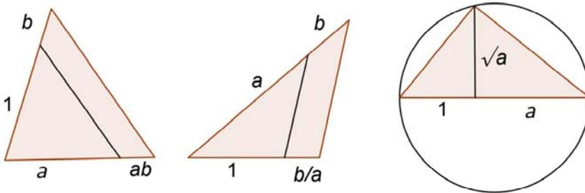
Figure 4: Constructions the line segment of lengths  $ab$ ,  $b/a$ ,  $\sqrt{a}$ .
